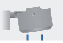
During the centrifugation run the buckets are swung out vertically  $\frown$
