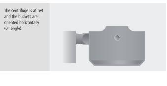
After the end of the centrifugation run, the buckets may not swing completely back to their original position (for example, due insufficiently lubricated rotor support bolts or asymmetric loading).
