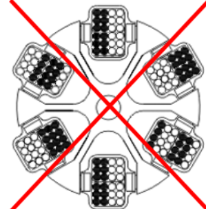
Fig. 16: Permissible and impermissible loading of an angle rotor and a swing-out rotor (example illustration)
