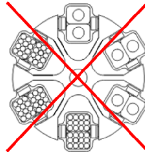
Fig. 15: Permissible and impermissible loading of a swing-out rotor with vessels of various sizes (example illustration)
