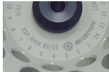
Fig. 7: Different service life – engraving on the bucket/rotor
