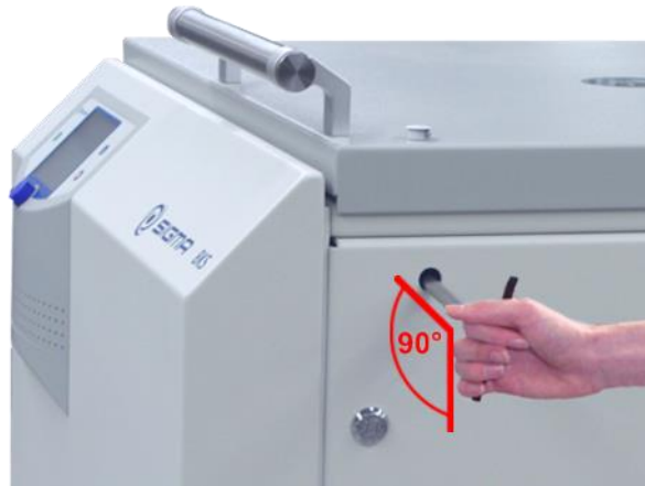
Fig. 41: The emergency lid release key must be inserted horizontally.
