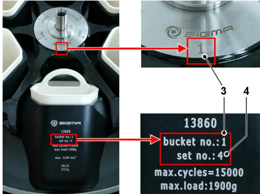
Fig. 9: The bucket number and set number on the bucket and the bucket number on the rotor
