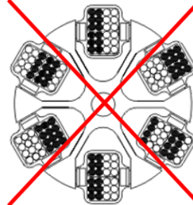
Fig. 12: Permissible and impermissible loading of an angle rotor and a swing-out rotor (example illustrations)
