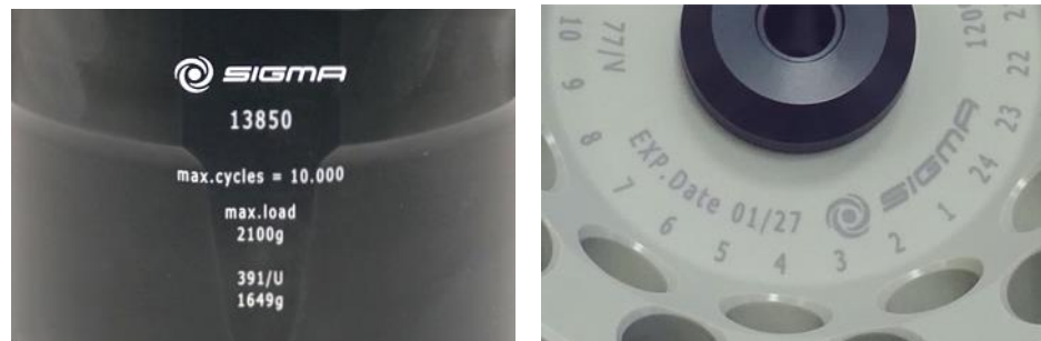
Fig. 6: Different service life – engraving on the bucket/rotor
