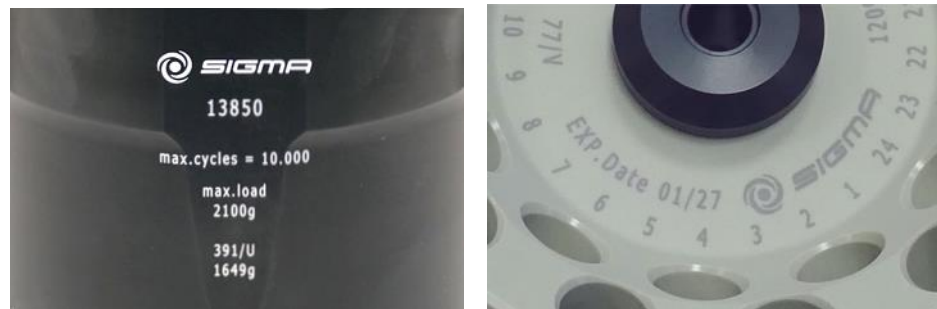
Fig. 5: Different service life – engraving on the bucket/rotor
