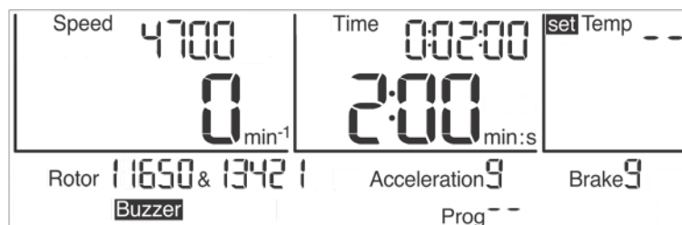
Fig. 22: Display with a deactivated temperature monitoring function
