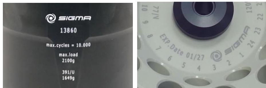
Fig. 6: Different service life – engraving on the bucket/rotor
