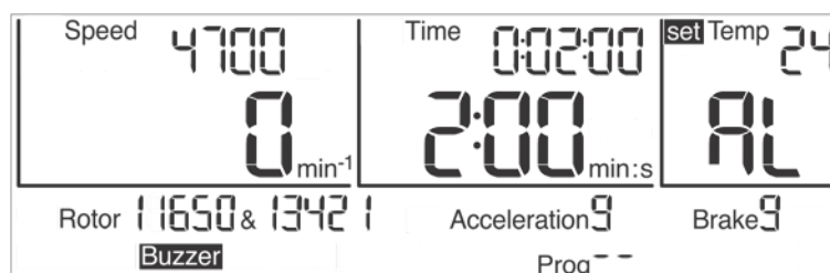
Fig. 23: Display with an activated temperature monitoring function
