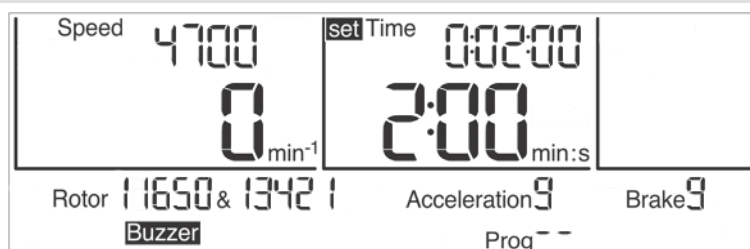
Fig. 18: Setting the runtime, here in the time unit "min:s"
