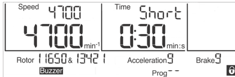
Fig. 21: Indication "Short" during a short run
