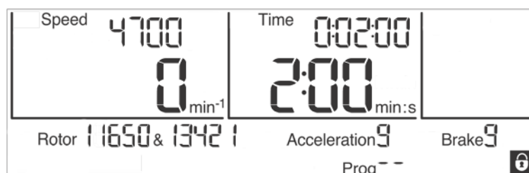
Fig. 32: "Padlock" symbol indicating an activated input lock
