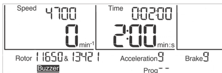
Fig. 28: The sound signal "Buzzer" is activated
