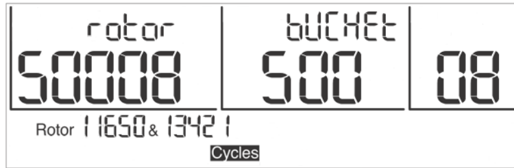
Fig. 31: Display when the maximum number of cycles is reached (flashing)
