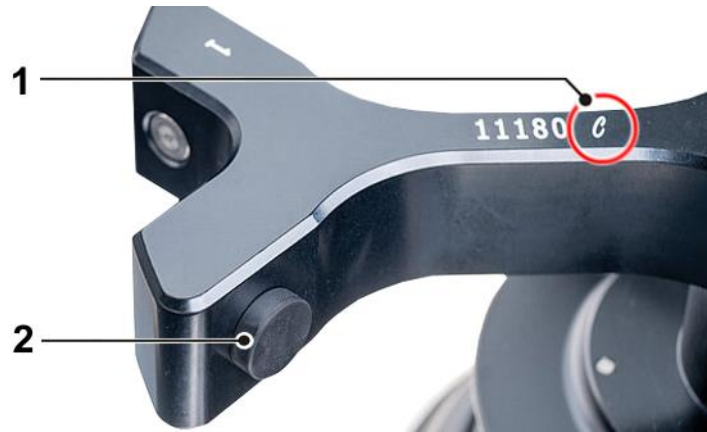
Fig. 7: Marking of a rotor with "Comfort" coating (example)
