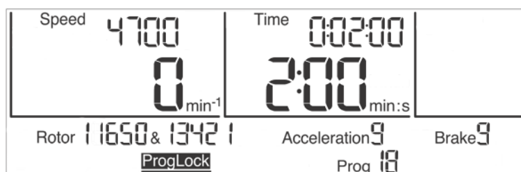
Fig. 29: The program lock "ProgLock" is activated
