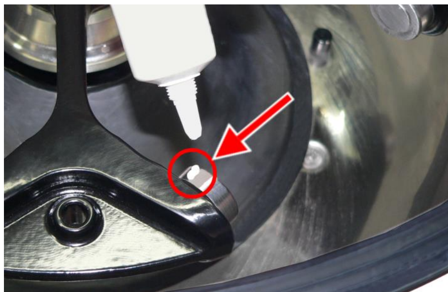
Fig. 37: Sufficient quantity of grease for one bolt
