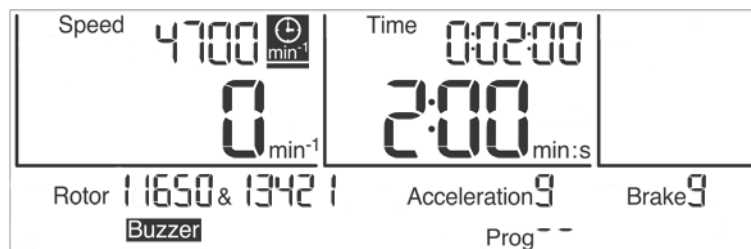
Fig. 19: The function "Runtime as of the set speed" is activated
