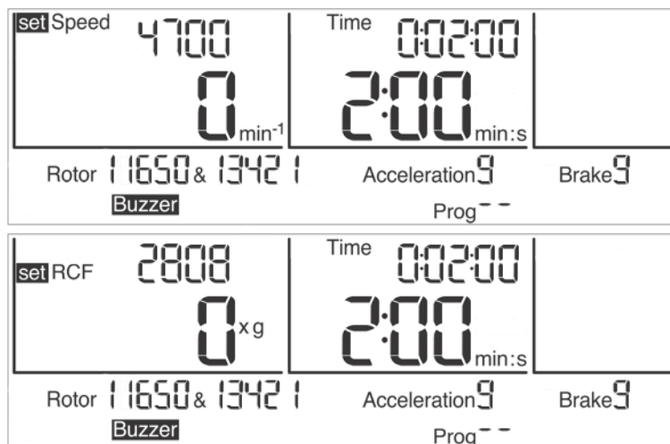
Fig. 17: Setting the speed value or the RCF value
