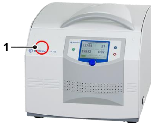
Fig. 33: Position of the opening for the emergency lid release
