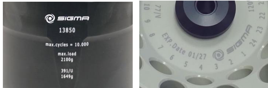
Fig. 5: Different service life – engraving on the bucket/rotor
