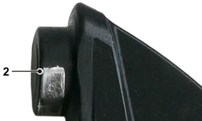
Fig. 7: Load-bearing bolt with completely worn-off coating – greasing required
