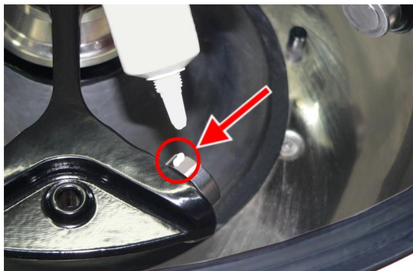
Fig. 34: Sufficient quantity of grease for one bolt
