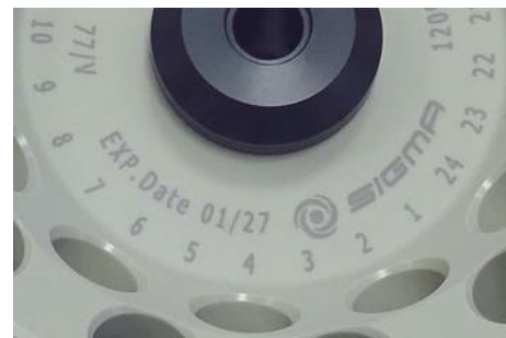
Fig. 4: Different service life – engraving on the bucket/rotor
