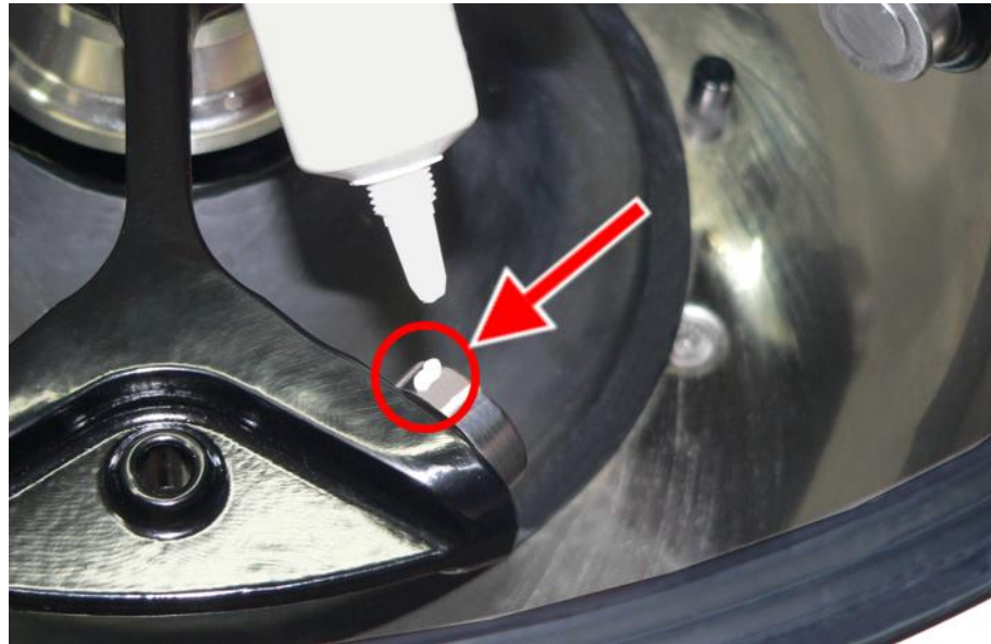
Fig. 16: Sufficient quantity of grease for one bolt
