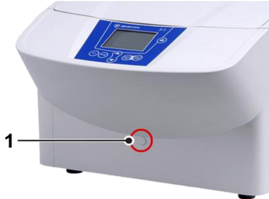
Fig. 23: Position of the opening for the emergency lid release
