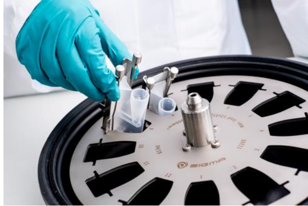
Fig. 13: Positioning the sample chamber system
