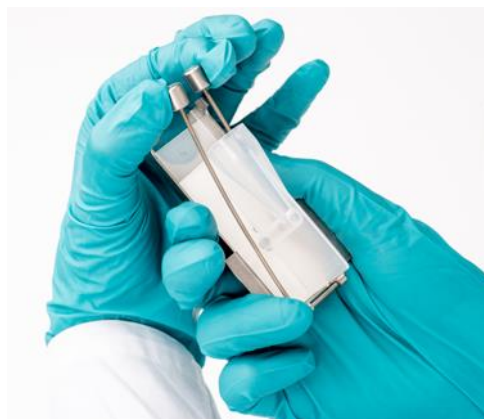
Fig. 12: Closing the clip
