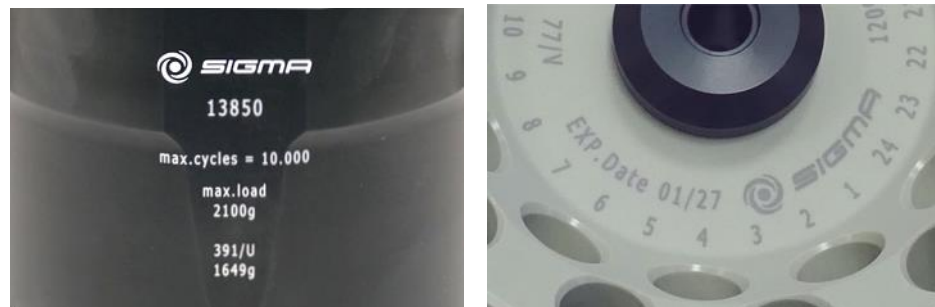
Fig. 5: Different service life – engraving on the bucket/rotor
