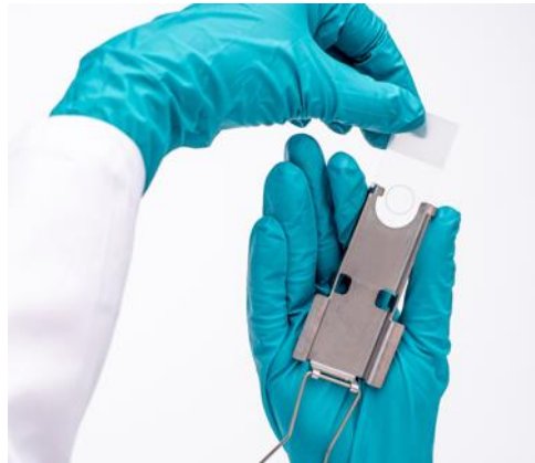
Fig. 10: Sliding the microscope slide into the clip
