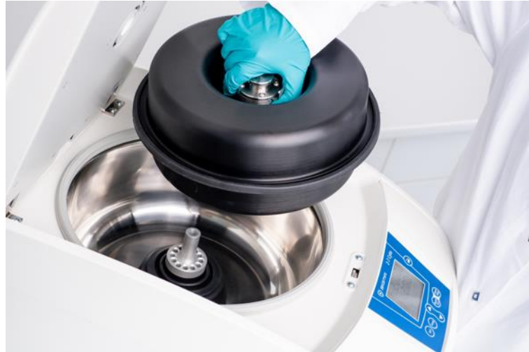
Fig. 15: Installing the cytology rotor
