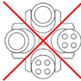
Fig. 18: Permissible and impermissible loading of a swing-out rotor with different tube sizes (example illustration)
