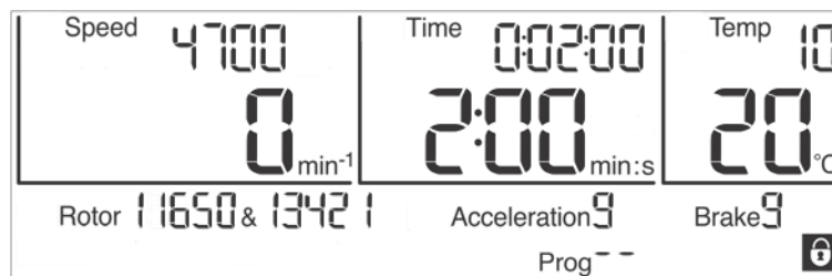
Fig. 28: "Padlock" symbol indicating an activated input lock
