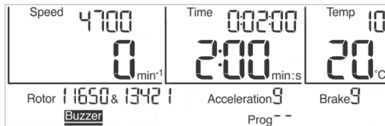
Fig. 24: The sound signal "Buzzer" is activated
