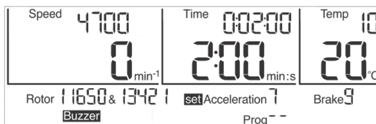
Fig. 22: Preselection of a curve; here: preselection of an acceleration curve
