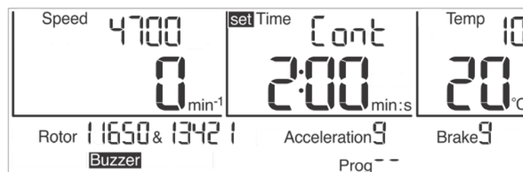
Fig. 17: Indication "Cont" during a continuous run
