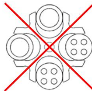
Fig. 9: Permissible and impermissible loading of a swing-out rotor with vessels of various sizes (example illustration)
