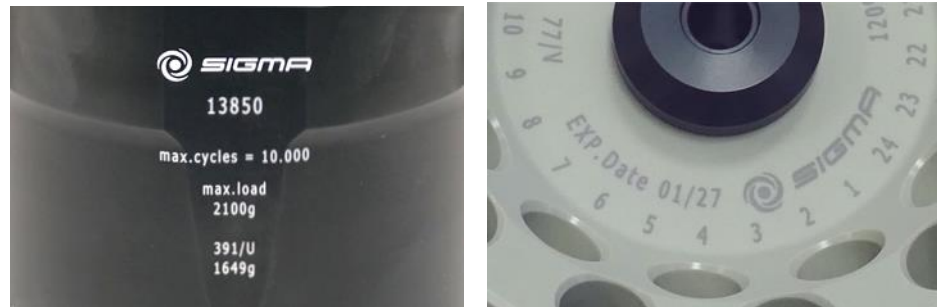
Fig. 4: Different service life – engraving on the bucket/rotor
