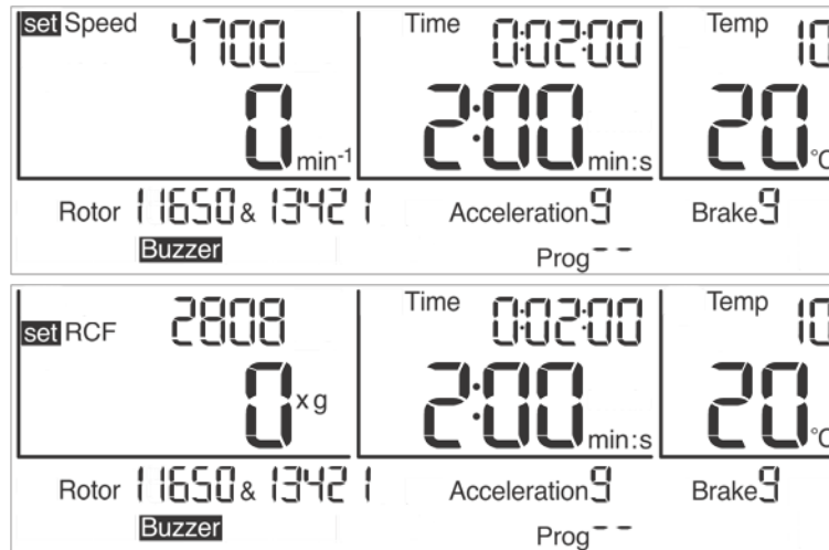
Fig. 14: Setting the speed value or the RCF value
