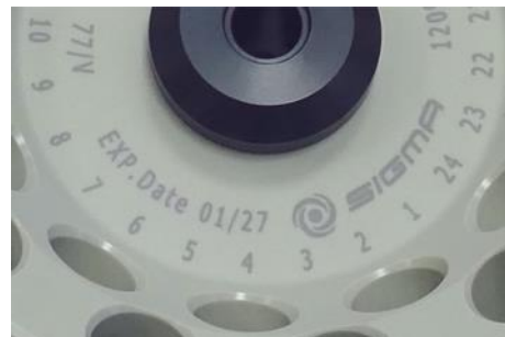
Fig. 4: Different service life – engraving on the bucket/rotor
