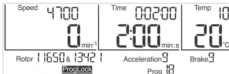
Fig. 25: The program lock "ProgLock" is activated
