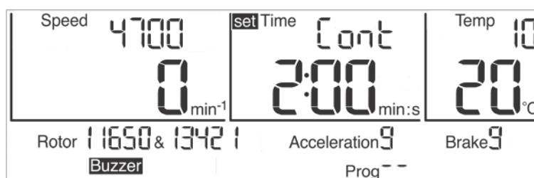
Fig. 17: Indication "Cont" during a continuous run
