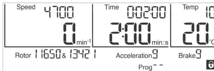
Fig. 28: "Padlock" symbol indicating an activated input lock
