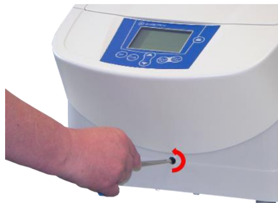
Fig. 9: Manual release of the lid lock
